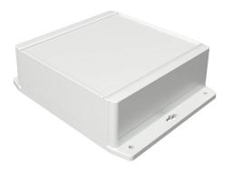
Hammond enclosure, NEMA 4/4X/6/6P/12/13, 180 x 180 x 65mm (HxWxD), integral mounting flange, ABS plastic, RAL 7035 light gray, screw cover, purchase subpanel separately.
