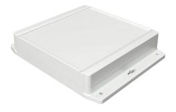
Hammond enclosure, NEMA 4/4X/6/6P/12/13, 180 x 180 x 40mm (HxWxD), integral mounting flange, ABS plastic, RAL 7035 light gray, screw cover, purchase subpanel separately.
