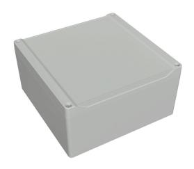
Hammond enclosure, NEMA 4/4X/6/6P/12/13, 180 x 180 x 90mm (HxWxD), ABS plastic, RAL 7035 light gray, screw cover with smooth recess, purchase subpanel separately.
