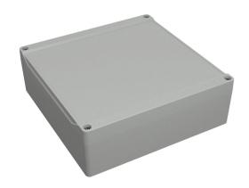
Hammond enclosure, NEMA 4/4X/6/6P/12/13, 180 x 180 x 60mm (HxWxD), polycarbonate, RAL 7035 light gray, screw cover with smooth recess, purchase subpanel separately.
