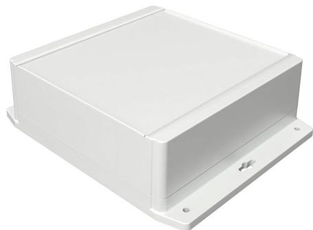
Hammond enclosure, NEMA 4/4X/6/6P/12/13, 180 x 180 x 65mm (HxWxD), integral mounting flange, polycarbonate, RAL 7035 light gray, screw cover, purchase subpanel separately.
