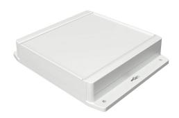
Hammond enclosure, NEMA 4/4X/6/6P/12/13, 180 x 180 x 40mm (HxWxD), integral mounting flange, polycarbonate, RAL 7035 light gray, screw cover, purchase subpanel separately.
