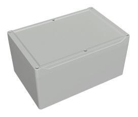
Hammond enclosure, NEMA 4/4X/6/6P/12/13, 240 x 160 x 120mm (HxWxD), ABS plastic, RAL 7035 light gray, screw cover with smooth recess, purchase subpanel separately.
