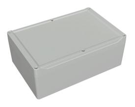
Hammond enclosure, NEMA 4/4X/6/6P/12/13, 240 x 160 x 90mm (HxWxD), ABS plastic, RAL 7035 light gray, screw cover with smooth recess, purchase subpanel separately.
