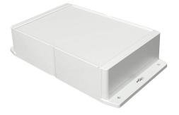
Hammond enclosure, NEMA 4/4X/6/6P/12/13, 240 x 160 x 62mm (HxWxD), integral mounting flange, ABS plastic, RAL 7035 light gray, screw cover, purchase subpanel separately.
