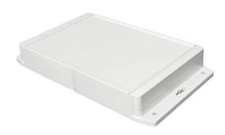
Hammond enclosure, NEMA 4/4X/6/6P/12/13, 240 x 160 x 37mm (HxWxD), integral mounting flange, ABS plastic, RAL 7035 light gray, screw cover, purchase subpanel separately.
