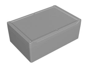
Hammond enclosure, NEMA 4/4X/6/6P/12/13, 240 x 160 x 90mm (HxWxD), polycarbonate, RAL 7035 light gray, screw cover with smooth recess, purchase subpanel separately.
