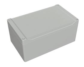
Hammond enclosure, NEMA 4/4X/6/6P/12/13, 200 x 120 x 91mm (HxWxD), ABS plastic, RAL 7035 light gray, screw cover with smooth recess, purchase subpanel separately.
