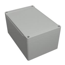
Hammond enclosure, NEMA 4/4X/6/6P/12/13, 180 x 120 x 91mm (HxWxD), polycarbonate, RAL 7035 light gray, screw cover with smooth recess, purchase subpanel separately.
