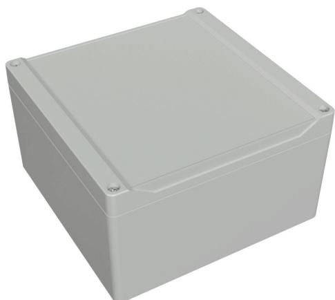
Hammond enclosure, NEMA 4/4X/6/6P/12/13, 160 x 160 x 91mm (HxWxD), ABS plastic, RAL 7035 light gray, screw cover with smooth recess, purchase subpanel separately.
