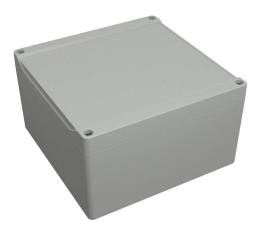
Hammond enclosure, NEMA 4/4X/6/6P/12/13, 160 x 160 x 91mm (HxWxD), polycarbonate, RAL 7035 light gray, screw cover with smooth recess, purchase subpanel separately.
