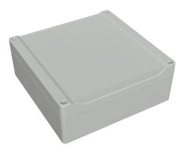
Hammond enclosure, NEMA 4/4X/6/6P/12/13, 160 x 160 x 61mm (HxWxD), ABS plastic, RAL 7035 light gray, screw cover with smooth recess, purchase subpanel separately.
