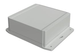
Hammond enclosure, NEMA 4/4X/6/6P/12/13, 160 x 160 x 63mm (HxWxD), integral mounting flange, ABS plastic, RAL 7035 light gray, screw cover, purchase subpanel separately.
