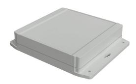
Hammond enclosure, NEMA 4/4X/6/6P/12/13, 161 x 160 x 38mm (HxWxD), integral mounting flange, ABS plastic, RAL 7035 light gray, screw cover, purchase subpanel separately.
