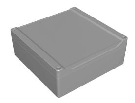
Hammond enclosure, NEMA 4/4X/6/6P/12/13, 160 x 160 x 61mm (HxWxD), polycarbonate, RAL 7035 light gray, screw cover with smooth recess, purchase subpanel separately.
