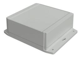
Hammond enclosure, NEMA 4/4X/6/6P/12/13, 160 x 160 x 63mm (HxWxD), integral mounting flange, polycarbonate, RAL 7035 light gray, screw cover, purchase subpanel separately.
