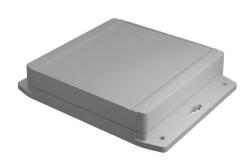
Hammond enclosure, NEMA 4/4X/6/6P/12/13, 161 x 160 x 38mm (HxWxD), integral mounting flange, polycarbonate, RAL 7035 light gray, screw cover, purchase subpanel separately.
