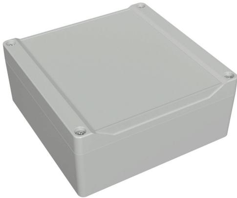
Hammond enclosure, NEMA 4/4X/6/6P/12/13, 140 x 140 x 60mm (HxWxD), ABS plastic, RAL 7035 light gray, screw cover with smooth recess, purchase subpanel separately.
