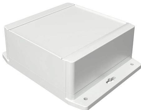
Hammond enclosure, NEMA 4/4X/6/6P/12/13, 140 x 140 x 62mm (HxWxD), integral mounting flange, ABS plastic, RAL 7035 light gray, screw cover, purchase subpanel separately.
