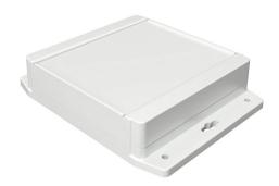
Hammond enclosure, NEMA 4/4X/6/6P/12/13, 140 x 140 x 37mm (HxWxD), integral mounting flange, ABS plastic, RAL 7035 light gray, screw cover, purchase subpanel separately.
