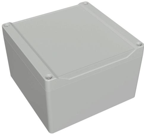
Hammond enclosure, NEMA 4/4X/6/6P/12/13, 140 x 140 x 90mm (HxWxD), ABS plastic, RAL 7035 light gray, screw cover with smooth recess, purchase subpanel separately.
