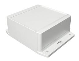
Hammond enclosure, NEMA 4/4X/6/6P/12/13, 140 x 140 x 62mm (HxWxD), integral mounting flange, polycarbonate, RAL 7035 light gray, screw cover, purchase subpanel separately.
