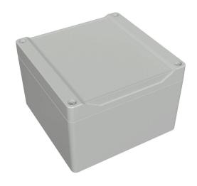
Hammond enclosure, NEMA 4/4X/6/6P/12/13,  $120 \times 120 \times 80$ mm (HxWxD), ABS plastic, RAL 7035 light gray, screw cover with smooth recess, purchase subpanel separately.
