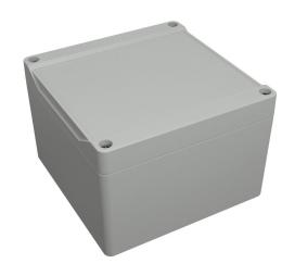
Hammond enclosure, NEMA 4/4X/6/6P/12/13, 120 x 120 x 80mm (HxWxD), polycarbonate, RAL 7035 light gray, screw cover with smooth recess, purchase subpanel separately.
