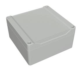
Hammond enclosure, NEMA 4/4X/6/6P/12/13,  $120 \times 120 \times 61$ mm (HxWxD), ABS plastic, RAL 7035 light gray, screw cover with smooth recess, purchase subpanel separately.
