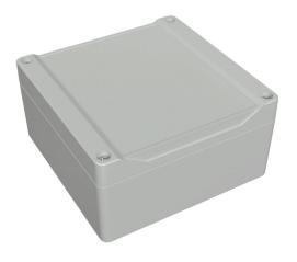
Hammond enclosure, NEMA 4/4X/6/6P/12/13, 120 x 120 x 61mm (HxWxD), ABS plastic, RAL 7035 light gray, screw cover with smooth recess, purchase subpanel separately.
