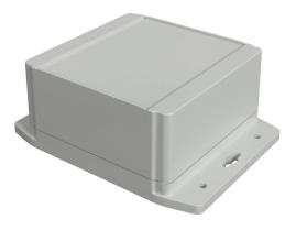
Hammond enclosure, NEMA 4/4X/6/6P/12/13, 121 x 120 x 63mm (HxWxD), integral mounting flange, ABS plastic, RAL 7035 light gray, screw cover, purchase subpanel separately.
