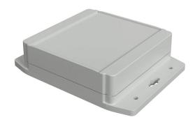
Hammond enclosure, NEMA 4/4X/6/6P/12/13, 121 x 120 x 38mm (HxWxD), integral mounting flange, ABS plastic, RAL 7035 light gray, screw cover, purchase subpanel separately.
