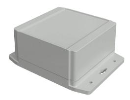
Hammond enclosure, NEMA 4/4X/6/6P/12/13, 121 x 120 x 63mm (HxWxD), integral mounting flange, polycarbonate, RAL 7035 light gray, screw cover, purchase subpanel separately.
