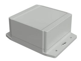
Hammond enclosure, NEMA 4/4X/6/6P/12/13, 121 x 120 x 63mm (HxWxD), integral mounting flange, polycarbonate, RAL 7035 light gray, screw cover, purchase subpanel separately.
