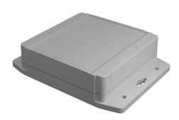
Hammond enclosure, NEMA 4/4X/6/6P/12/13, 121 x 120 x 38mm (HxWxD), integral mounting flange, polycarbonate, RAL 7035 light gray, screw cover, purchase subpanel separately.
