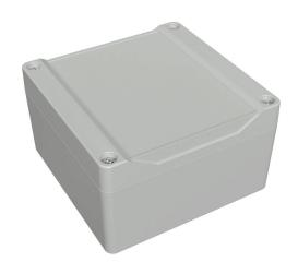
Hammond enclosure, NEMA 4/4X/6/6P/12/13,  $105 \times 105 \times 60$ mm (HxWxD), ABS plastic, RAL 7035 light gray, screw cover with smooth recess, purchase subpanel separately.
