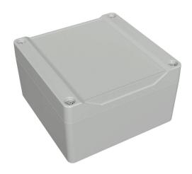
Hammond enclosure, NEMA 4/4X/6/6P/12/13, 105 x 105 x 60mm (HxWxD), ABS plastic, RAL 7035 light gray, screw cover with smooth recess, purchase subpanel separately.
