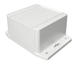
Hammond enclosure, NEMA 4/4X/6/6P/12/13, 105 x 105 x 62mm (HxWxD), integral mounting flange, ABS plastic, RAL 7035 light gray, screw cover, purchase subpanel separately.
