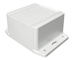
Hammond enclosure, NEMA 4/4X/6/6P/12/13, 105 x 105 x 62mm (HxWxD), integral mounting flange, ABS plastic, RAL 7035 light gray, screw cover, purchase subpanel separately.
