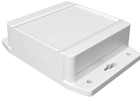
Hammond enclosure, NEMA 4/4X/6/6P/12/13, 105 x 105 x 37mm (HxWxD), integral mounting flange, ABS plastic, RAL 7035 light gray, screw cover, purchase subpanel separately.
