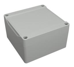
Hammond enclosure, NEMA 4/4X/6/6P/12/13, 105 x 105 x 60mm (HxWxD), polycarbonate, RAL 7035 light gray, screw cover with smooth recess, purchase subpanel separately.
