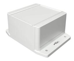
Hammond enclosure, NEMA 4/4X/6/6P/12/13, 105 x 105 x 62mm (HxWxD), integral mounting flange, polycarbonate, RAL 7035 light gray, screw cover, purchase subpanel separately.
