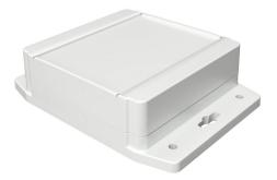
Hammond enclosure, NEMA 4/4X/6/6P/12/13, 105 x 105 x 37mm (HxWxD), integral mounting flange, polycarbonate, RAL 7035 light gray, screw cover, purchase subpanel separately.
