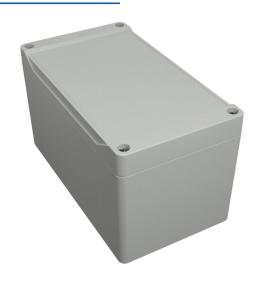
Hammond enclosure, NEMA 4/4X/6/6P/12/13,  $160 \times 90 \times 91$ mm (HxWxD), polycarbonate, RAL 7035 light gray, screw cover with smooth recess, purchase subpanel separately.
