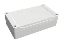
Hammond enclosure,  $160 \times 90 \times 46 \text{mm}$  (HxWxD), ABS plastic, RAL 7035 light gray, screw cover with smooth recess, purchase subpanel separately.
