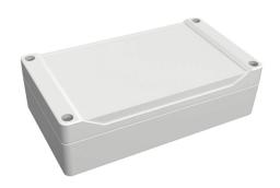
Hammond enclosure, NEMA 4/4X/6/6P/12/13, 160 x 90 x 46mm (HxWxD), polycarbonate, RAL 7035 light gray, screw cover with smooth recess, purchase subpanel separately.
