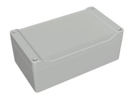
Hammond enclosure, NEMA 4/4X/6/6P/12/13, 160 x 90 x 61mm (HxWxD), ABS plastic, RAL 7035 light gray, screw cover with smooth recess, purchase subpanel separately.
