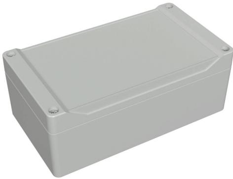
Hammond enclosure, NEMA 4/4X/6/6P/12/13, 160 x 90 x 61mm (HxWxD), ABS plastic, RAL 7035 light gray, screw cover with smooth recess, purchase subpanel separately.
