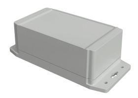
Hammond enclosure, NEMA 4/4X/6/6P/12/13, 160 x 91 x 63mm (HxWxD), integral mounting flange, ABS plastic, RAL 7035 light gray, screw cover, purchase subpanel separately.
