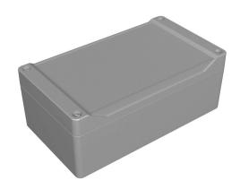
Hammond enclosure, NEMA 4/4X/6/6P/12/13, 160 x 90 x 61mm (HxWxD), polycarbonate, RAL 7035 light gray, screw cover with smooth recess, purchase subpanel separately.
