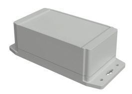
Hammond enclosure, NEMA 4/4X/6/6P/12/13, 160 x 91 x 63mm (HxWxD), integral mounting flange, polycarbonate, RAL 7035 light gray, screw cover, purchase subpanel separately.
