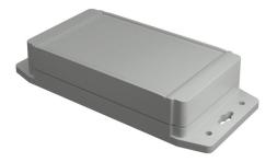
Hammond enclosure, NEMA 4/4X/6/6P/12/13, 160 x 91 x 38mm (HxWxD), integral mounting flange, polycarbonate, RAL 7035 light gray, screw cover, purchase subpanel separately.
