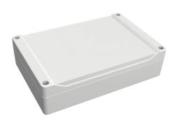
Hammond enclosure, NEMA 4/4X/6/6P/12/13, 180 x 120 x 46mm (HxWxD), polycarbonate, RAL 7035 light gray, screw cover with smooth recess, purchase subpanel separately.
