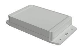
Hammond enclosure, NEMA 4/4X/6/6P/12/13, 180 x 121 x 38mm (HxWxD), integral mounting flange, ABS plastic, RAL 7035 light gray, screw cover, purchase subpanel separately.
