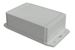
Hammond enclosure, NEMA 4/4X/6/6P/12/13, 180 x 121 x 62mm (HxWxD), integral mounting flange, polycarbonate, RAL 7035 light gray, screw cover, purchase subpanel separately.
